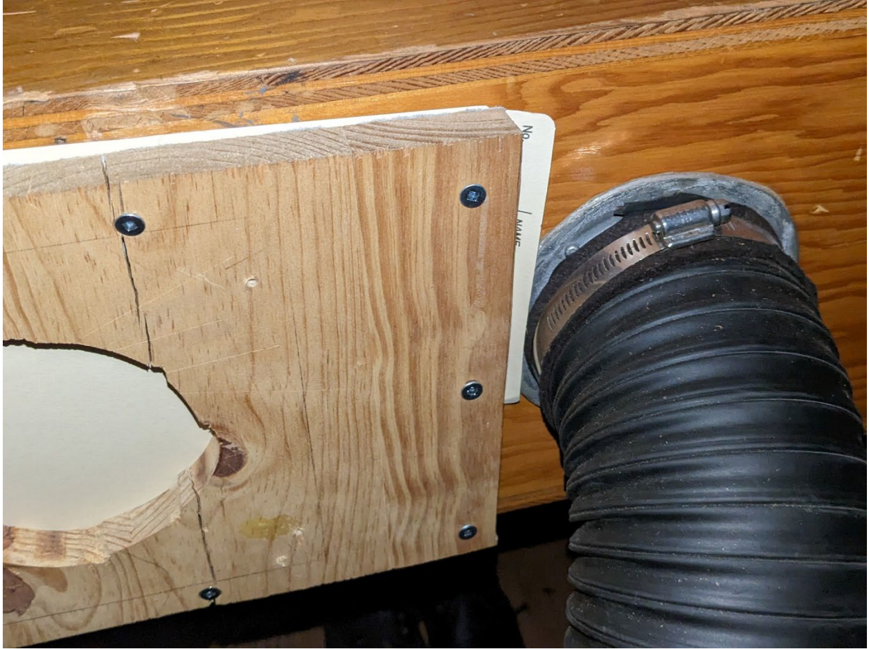
Figure 5: A repair to a wind trunk made with a file folder and plank of wood leftover from a nearby repair.
