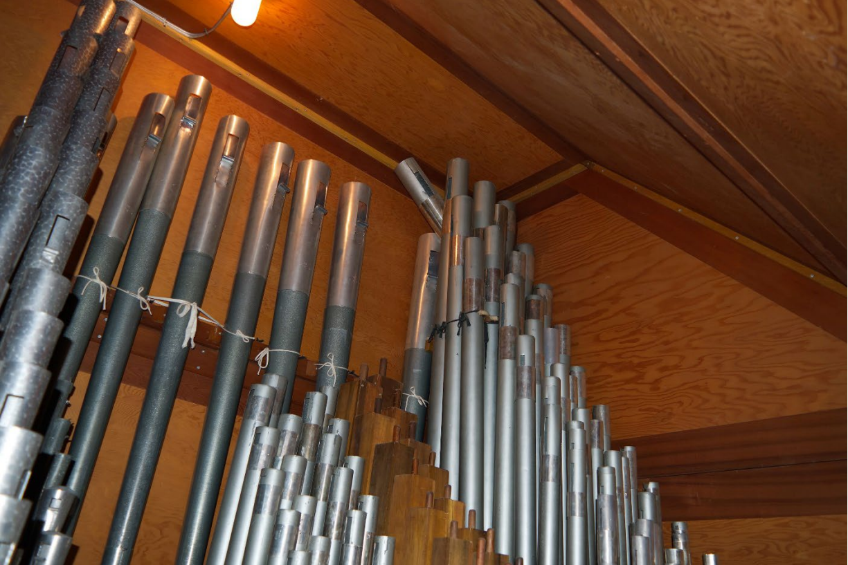
Figure 3: Unsupported and cramped larger pipes in the Swell Organ chest.
